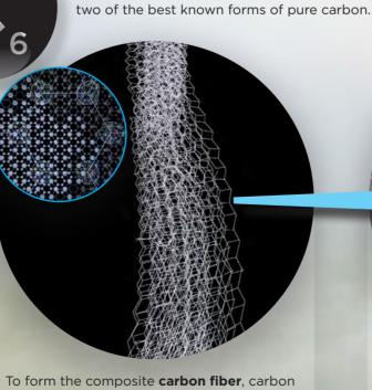
atoms are formed into crystalline chains. These extremely fine filaments are then twisted into fibers called threads which in turn are woven together and mixed with epoxy resin to form a material called a tape.
