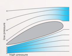
Bernoulli's Principle: Developed by Swiss mathematician Daniel Bernoulli, this principle states that the pressure of a flowing fluid or gas decreases as the velocity increases and increases as the velocity decreases.
