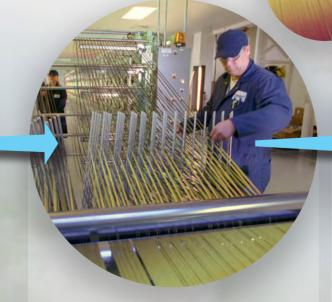
Through an intricate process of weaving, layering, mixing with resin, pressing and cooking with heat and pressure (in an autoclave)—carbon fiber tape is formed into specific composite components for the
