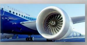
Jet Turbine. Jet turbine engines push air through the blades of a spinning turbine, which compresses the air. Fuel is then combined with the air and ignited. When the fuel burns, it rapidly expands from liquid to a gas and is forced out the rear of the engine. As the gas is forced out, the airplane is pushed forward.
