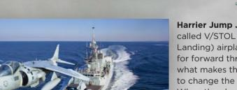
Harrier Jump Jet. These amazing aircraft are called V/STOL (Vertical/Short Take-Off and Landing) airplanes. They use jet turbine engines for forward thrust, just like a standard jet. But what makes these planes special is their ability to change the direction of their jet nozzles. When they land and take off, their jets can be pointed straight down, allowing the jump jet to lift straight off the ground. Harriers can even hover like hummingbirds.
